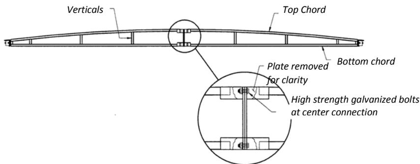
Strong, robust, galvanized square hollow section tube construction used for bottom chord as well as top chord of truss and also for verticals
