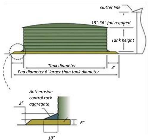
Inert rock aggregate must be placed around the base (circumference) of your tank after installation. Failure to do so will void all applicable warranties.\* It is recommended that a load of water (a minimum of 2600 gallons) be delivered at the completion of construction. If, however, your tank has been left empty for any period of time, please contact either Acer Water Tanks or your local installer.
