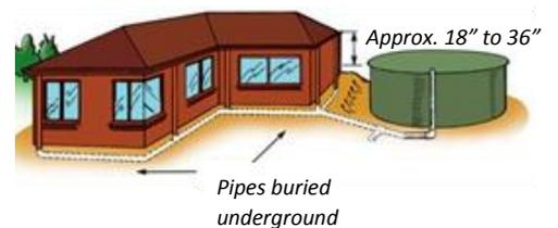
This is the most popular method of rainwater collection because of its neat appearance. Water is channeled via PVC water pipe below ground and up into the tank through the filter basket. It is important that the tank entry point is a minimum 18 inches lower than the roof gutter and that the PVC pipe is sealed and watertight. Please note, the farther the tank is from the house, the greater the height differential required.
