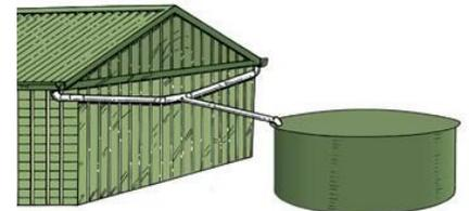
All PVC water pipes are channeled through the filter basket mounted on the roof of the water tank.
